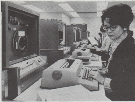
Typewriters linked to magnetic tape storage units. Taped information can then be reorganised for computer typesetting.
