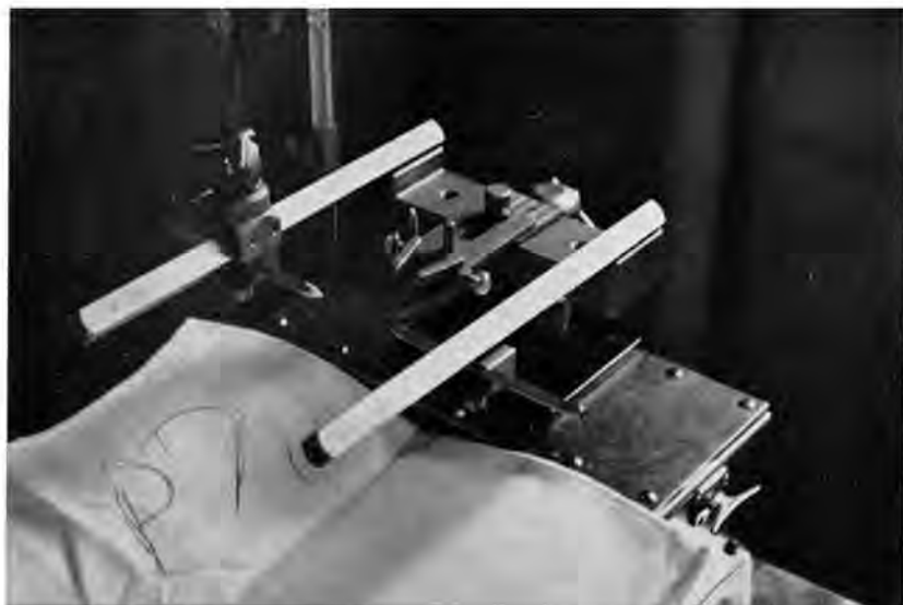
Fig. 4. Stereotaxic surgical instrument for implanting electrodes in the animal brain. The animal is anesthetized and his head securely mounted between the two large guide bars. Using calibrated electrode carriers, one of which is shown attached to the left guide bar, needle electrodes can be lowered into the brain through small drill holes made in the skull. Two electrodes are shown on the towel under the instrument, another is mounted in the carrier.
