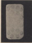
d) 2.8 mm x 1.4 mm Conductor 18 Strands T48 in OFHC Copper Matrix 735 a at 75 kG
