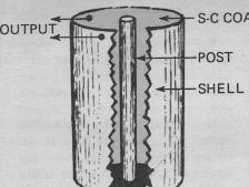
post in the center of the shell is coated with a low-energy betaemitting radioactive isotope-one of such low energy that an inch or so of air stops the radiation completely. The semiconductor coating serves simply as a beta-ray detector.
