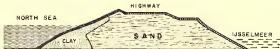
Cross section through the big dam across the mouth of the (former) Zuider Zee.
